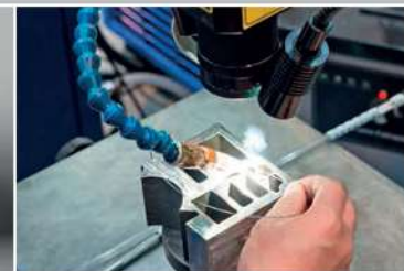
Nozzle for Argon gas Ugello per gas Argon
